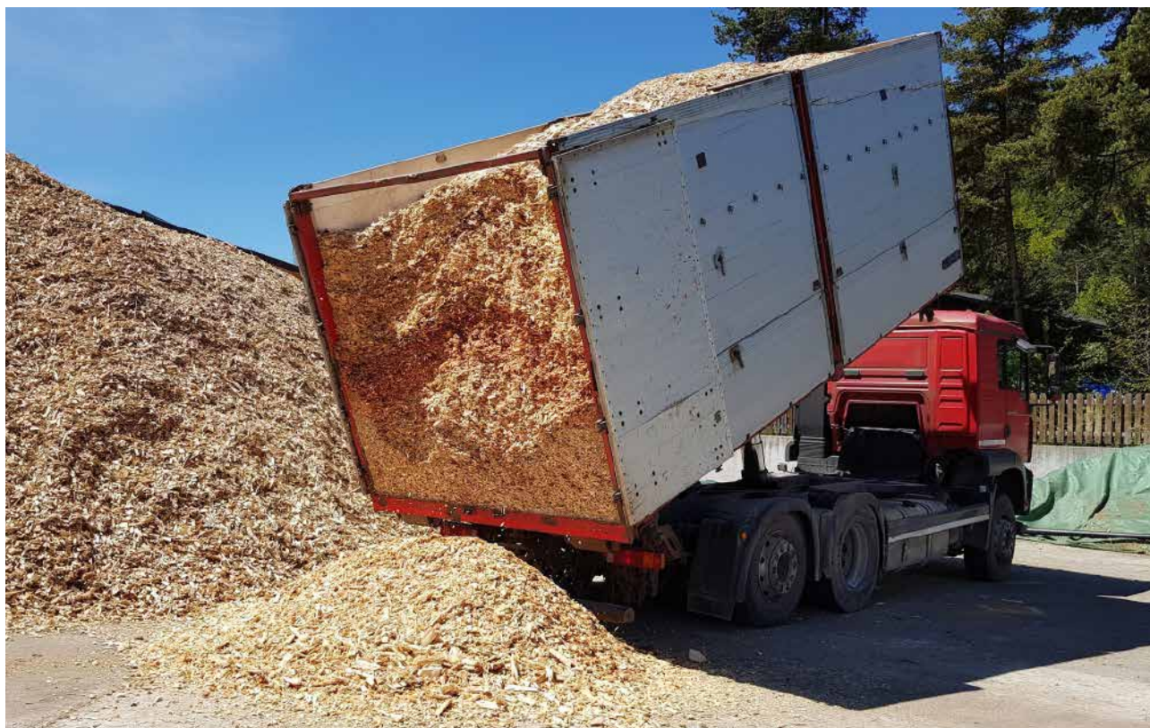
Delivery of woodchips from forest biomass at a district heating plant in South Tyrol, Italy. Source: ETA Florence
